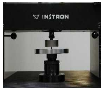
Universal Machine for compression strength test
